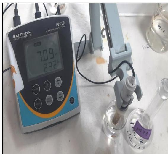
**Fig: Glass electrode and pH meter**
